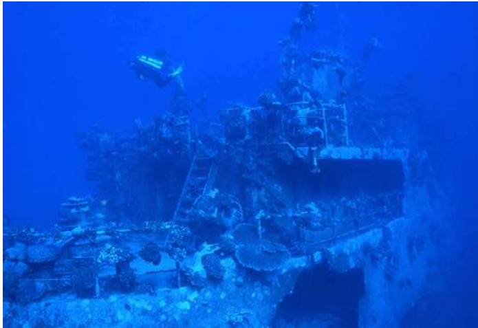
A diver hovers over the stern of the Moma class Surveillance vessel at Zabagad Island .The damage from the explosion can clearly be seen in the starboard hull.On the aft deck are the winches for towing the sonar arrays.
